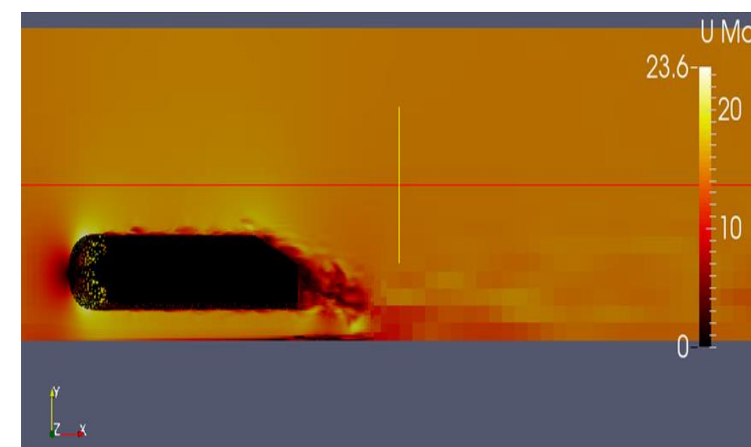
Figure 5: X direction velocity contours for case with 8 vortex generators
